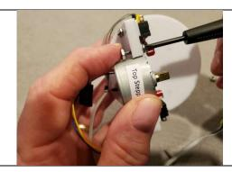
Fit the second screw and nut to secure the other side of the stepper motor. Note that the stepper motor is mounted on the same side as the limit switches.
