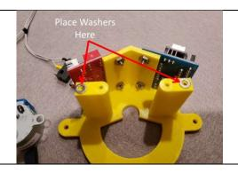
Place a stepper motor on the camera base as shown. The motor wires are routed behind the motor. Both motors are the same.
